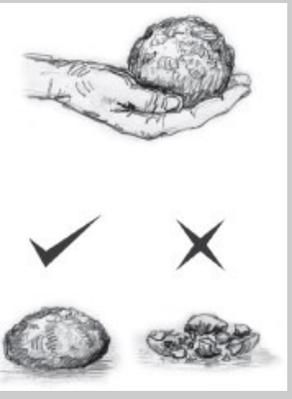
3. Drop the ball from head height onto flat ground. If the ball retains its shape, or goes only slightly out of shape, it has enough clay content and is thus good for pond construction. If the ball flattens out, crack open, or even shatter on impact to the ground, it's not good for pond construction.
